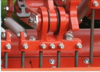
The robust tine holders with large sized ball bearings are capable of withstanding extreme conditions, such as jolts, dirt and sand.
