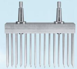
Solid tines 5 x 65, 5 x 135, 8 x 65 or 8 x 150 mm are mounted in the multi-tine holder "nail board". 24, 16 or 8 tines can be mounted, depending on the task and the required hole pattern. The "sandwich construction" of the nail board allows quick and easy tine replacement.
