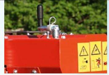
The working depth of the TERRA SPIKE® XF/XD can be adjusted easily and without tools by using a hand crank.
