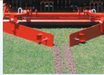
When using hollow tines the cores can be deposited in rows by means of the optional swathboard. This makes the subsequent collection of the cores much easier.
