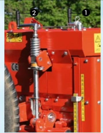
Central, quick adjustment of the tine entry angle (90 to 65°) and working depth without the need for tools. With only one central crank, you can easily and quickly make these settings which are so important for the quality of the work - regardless of the length of tine you have fitted or whether the tine is new or used.
